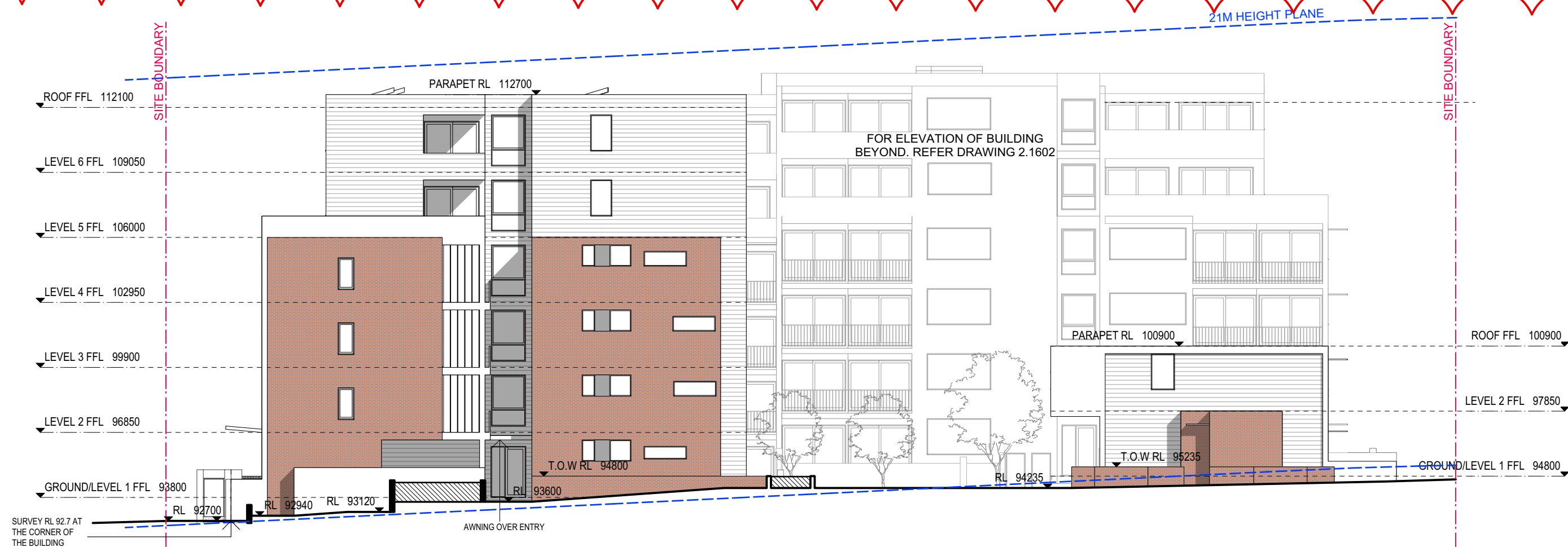
1 Internal Elevation East - Building E & F Scale: 1:200
